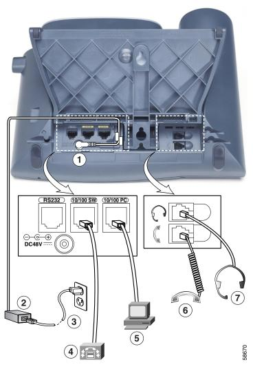
Figure 3-1 Cisco IP Phone Models 7960 and 7940 Cable Connections
